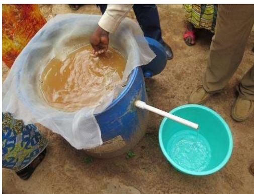
This simple system enables people to purify easily soiled water. Dirty water is filtered by a net and by sand. It requires very little materials.
